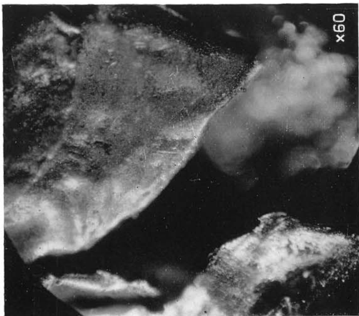
PLATE III (b). Hole in same specimen showing no fusion at edges.
